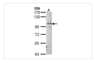
Sample (30 ug of whole cell lysate) A: Raji 7.5% SDS PAGE Primary antibody diluted at 1: 5000
