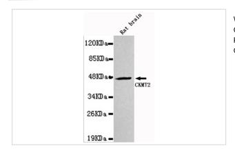
Western blot detection of CKMT2 in Rat Brain lysates using CKMT2 antibody (1:1000 diluted).
